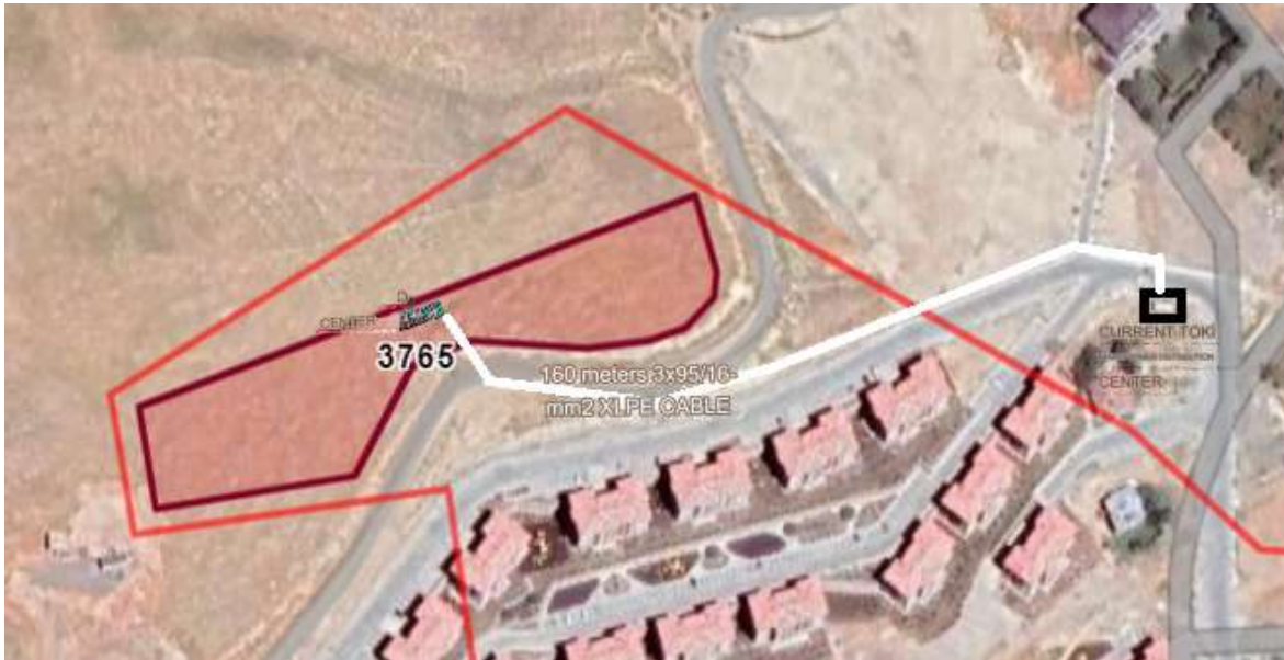
Figure 3. Energy Transmission Line
